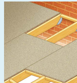
SE panels are laid with long edges in-line with the joists
