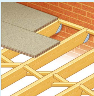
T&G panels are laid with long edges across the joists
