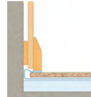
Vapour control layer without battened floor
